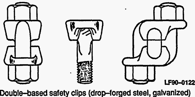
Figure 8-13. Double-based safety clips (drop-forged steel, galvanized).
