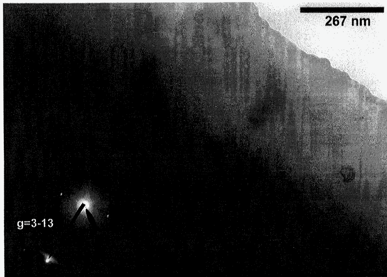
Figure 1.27: A bright field image for the two-beam condition, g=3-13 , shown in the inset. A change in contrast occurs for the precipitates relative to figure 1.28. The two-beam condition was obtained by tilting from the [-233] zone axis. Note that s is slightly negative.
