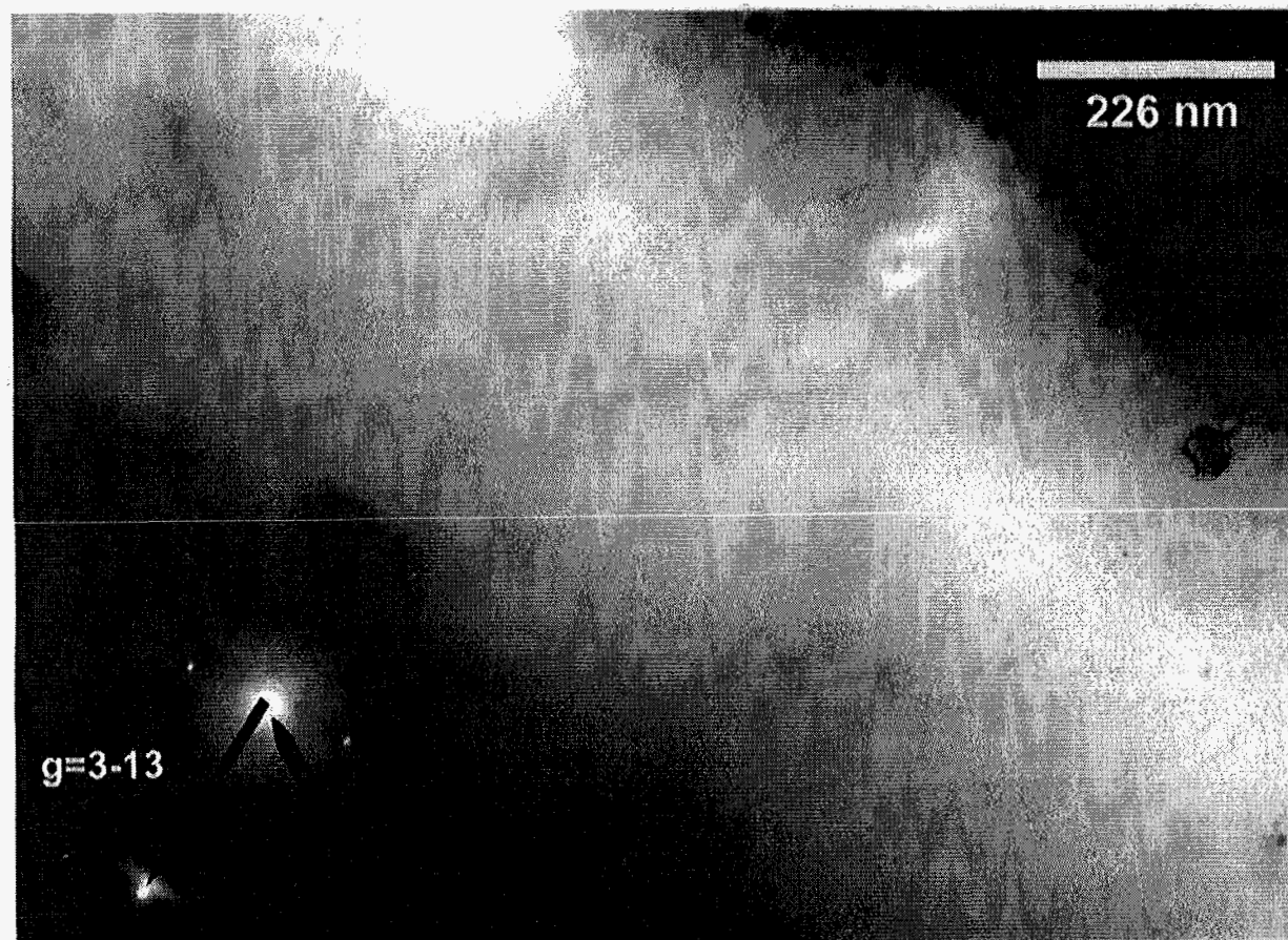
Figure 1.28: A dark field image for the two beam condition, g=3-13 , shown in the inset. A change in contrast occurs for the precipitates relative to figure 1.27.
