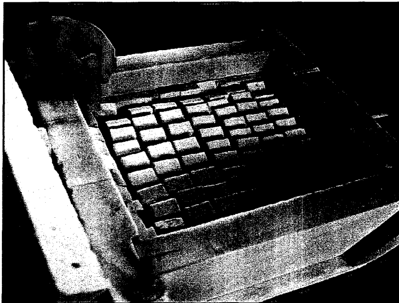
Figure 16. Photo showing the top layer (two total) of samples in which 125 samples (5.8 kg) nitrided using MW heating.
