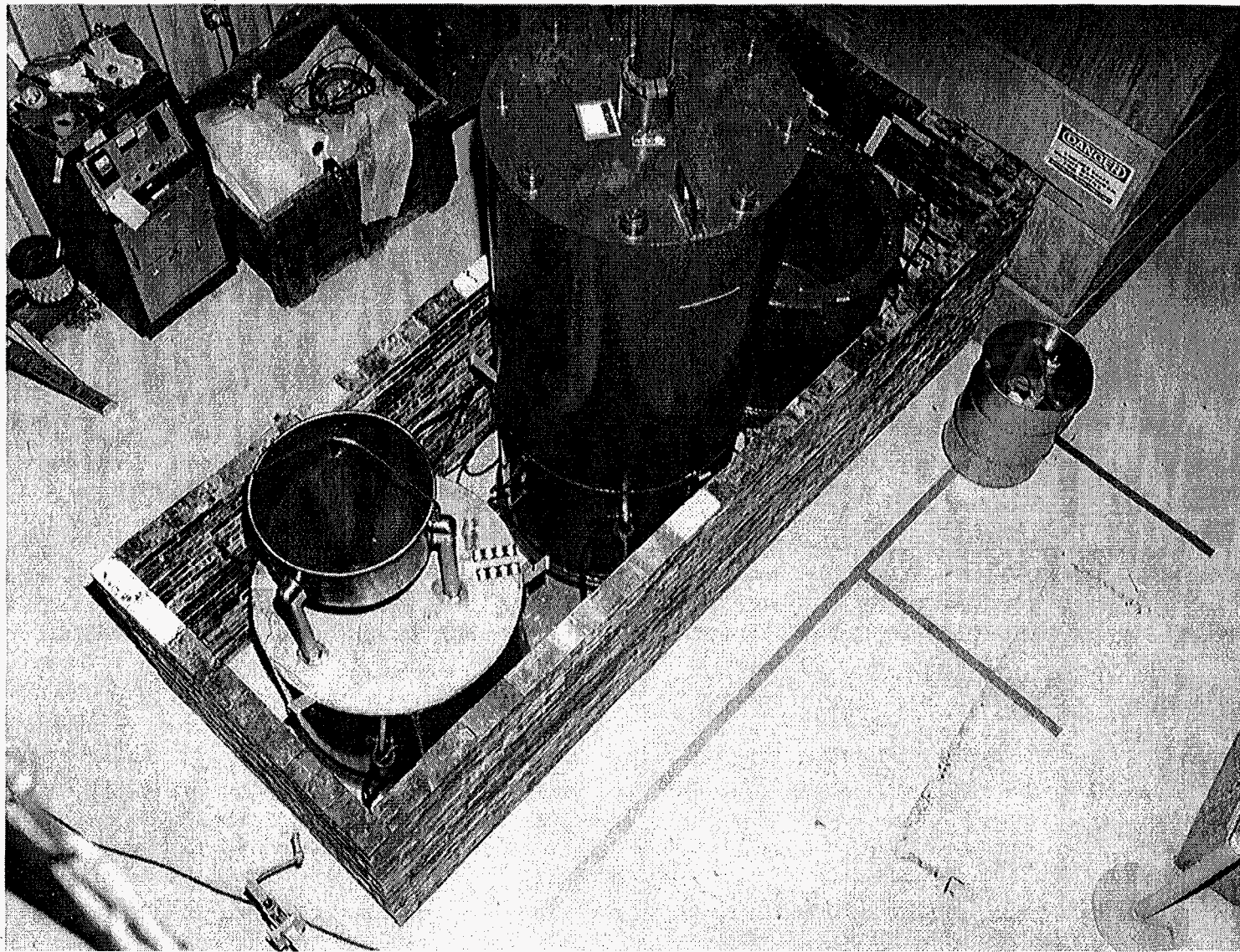
Fig. 17. Photograph showing shielded containers, shielded remote transfer bell, lead brick-shielded area, and remote vermiculite hopper for the CsRD.
