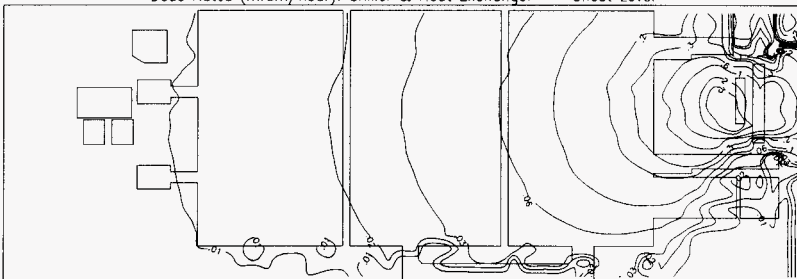
Dose Rates (mrem/hour): Chiller & Heat Exchanger -- Chest Level
