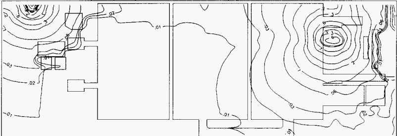
Dose Rates (mrem/hour): NW Filter Media & Pump #1 on East Side -- Knee Level
