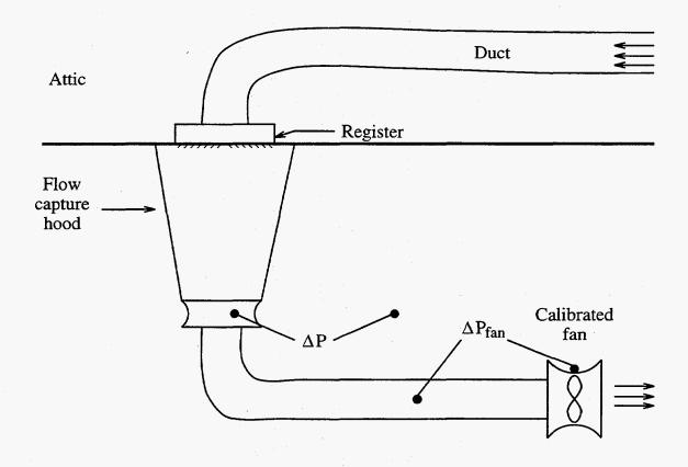
**FIGURE 1.** Arrangement of flow capture hood and calibrated fan demonstrating measurement of air flow out a supply register.
