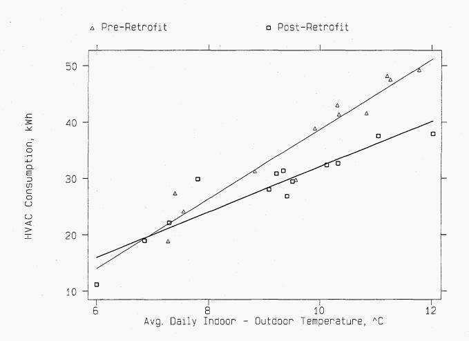
**FIGURE 4.** Daily heat-pump energy use as a function of average indoor-outdoor temperature differential before and after duct retrofit. Pre-retrofit regression line slope is 6 kWh/day  $^{o}$ C ( $R^{2}$  = 0.92), and whereas post retrofit is 4 kWh/day  $^{o}$ C ( $R^{2}$  = 0.86). Data for House 6.
