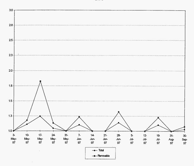
The chart above reflects actual data from 241-U Tank Farm. An indexed value of one indicates that all surveys performed were below the detection limits of the instruments. Surveys performed on 3 May, 31 May, 14 June, 21 June, 5 July, 12 July, and 31 August found no contamination. The indexed value for total contamination removable contamination is clearly higher than that for total. This indicates the contamination is primarily removable.
