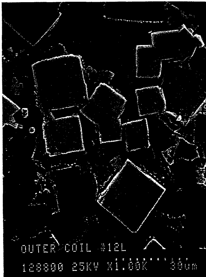
Fig. 3 Blocky Sb_2Sn_3 intermetallic compound particles.
