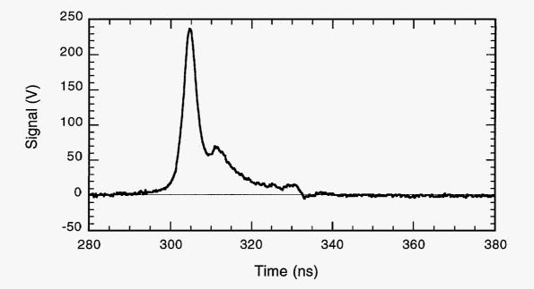
Fig. 5. A typical pulse from an x-ray detector showing the reflection caused by the insertion capacitor.
