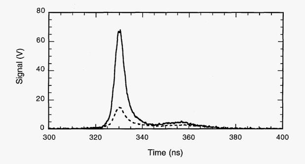
Fig. 7. A neutron-damaged PCD (dashed curve) is compared with an undamaged normal diamond PCD (solid curve).
