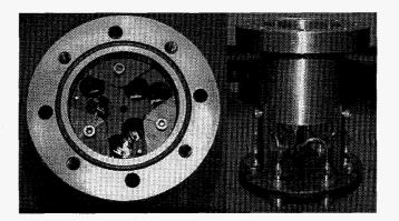
Fig. 2. The PCDs are mounted in a stainless steel housing that has integral x-ray filter holders and sweeper magnets.
