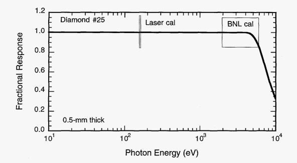
Fig. 6. Calibration data for Diamond Element # 25 is superimposed on a theoretical diamond absorption curve (scaled to unity). The size of the boxes are indicative of the calibration errors.
