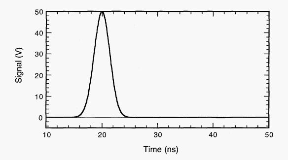
Fig. 4a. A pulse is generated by a variable resistance load on a biased 20-ns long 50- $\Omega$  cable and is measured as a voltage across a 50- $\Omega$  load.
