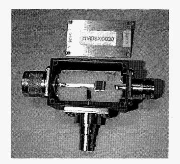
Fig. 3. The Sandia-designed insertion unit is shown. The DC blocking capacitor is mounted in a 50- $\Omega$  stripline configuration. A 100-k $\Omega$  resistor is used to place a DC bias voltage on the unit.
