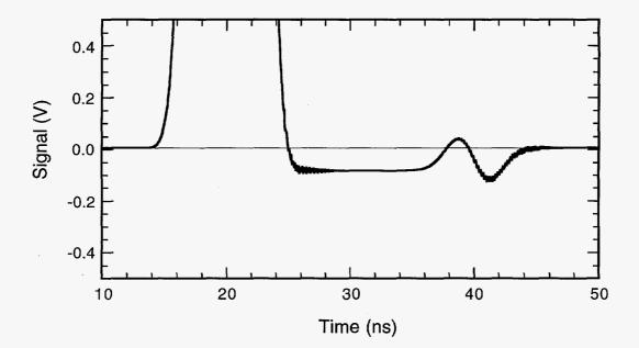
Fig. 4b. The same pulse in Fig. 3A is shown with the reflection caused by the capacitive insertion unit.
