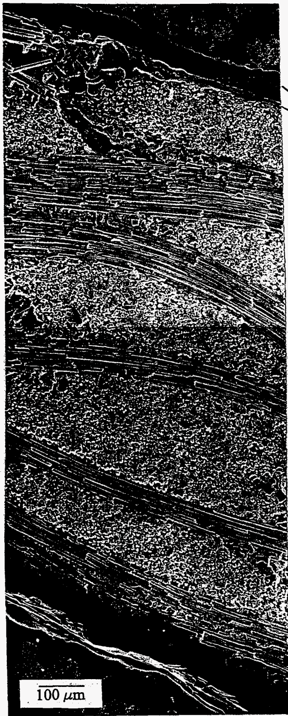
Figure 5. Cross section of a CMC tube
