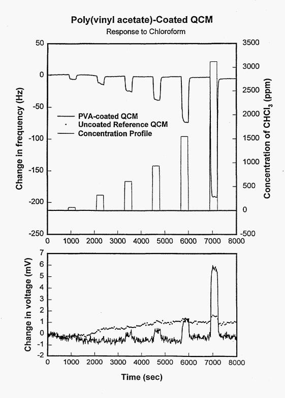
Figure 3. Top graph shows frequency response for a poly(vinyl acetate)-coated QCM (solid line) and an uncoated reference QCM (dotted line) to the indicated concentration profile of chloroform (dashed line). Bottom graph shows the damping voltage response.
