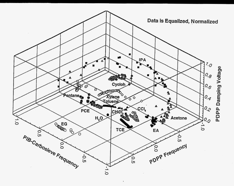
Figure 5. Representation of equalized and normalized data from two sensors (three total responses) showing clustering of data for each VOC and effective separation from other VOCs.
