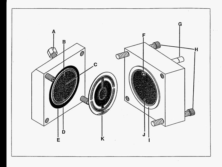
Figure 1. QCM liquid flow cell. (A) Zero dead volume tube connector. (B) Liquid exit port. (C) Liquid cavity. (D) Liquid inlet port. (E). O-ring. (F) Pogo pin rf-contact. (G) SMB rf-connector. (H) Socket Head Cap Screws. (I) Polycarbonate spacer. (J) Pogo pin ground contact. (K) QCM.
