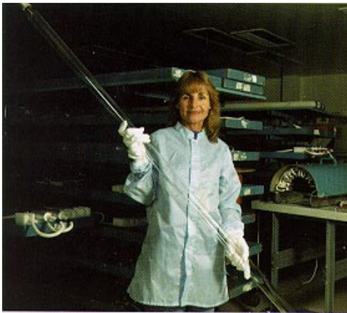
Figure 11. A 4.8 cm diameter, 2 meter long NIF flashlamp, one of approx. 8,000 in the laser amplifiers.
