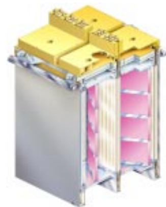
Figure 9. A section of an amplifier "bundle" consisting of eight laser apertures in two 4-high columns.
