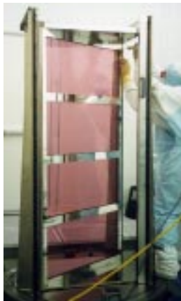
Figure 10. A slab cassette containing a four-high column of laser slabs that are inserted and removed from the amplifier as a unit.
