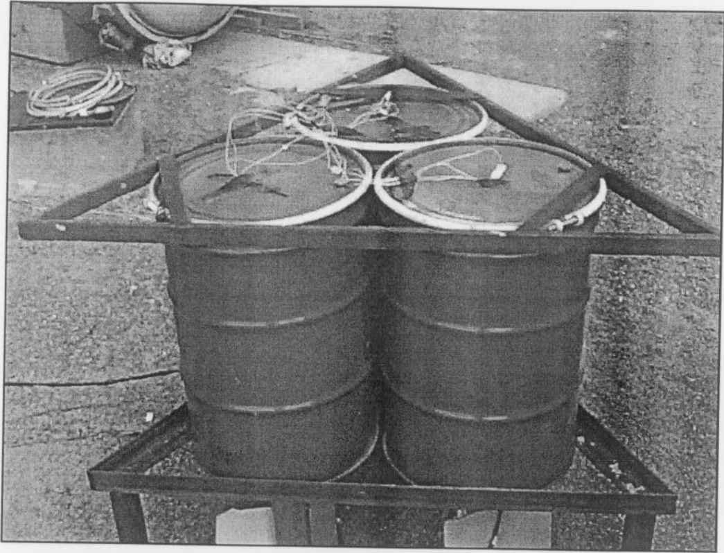
Figure 16. Three barrels on stand for 6(c) fire test. Thermocouple wires can be seen coming out of each lid
