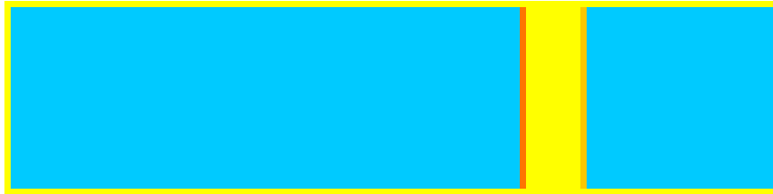
Figure 5: The initial configuration of the dense gas spherical shell shown in logical i and j coordinates. In this view, spherical shells appear as vertical lines. Yellow denotes full dense shell cells and blue denotes full light gas cells. The origin is the left edge of the computational domain.
