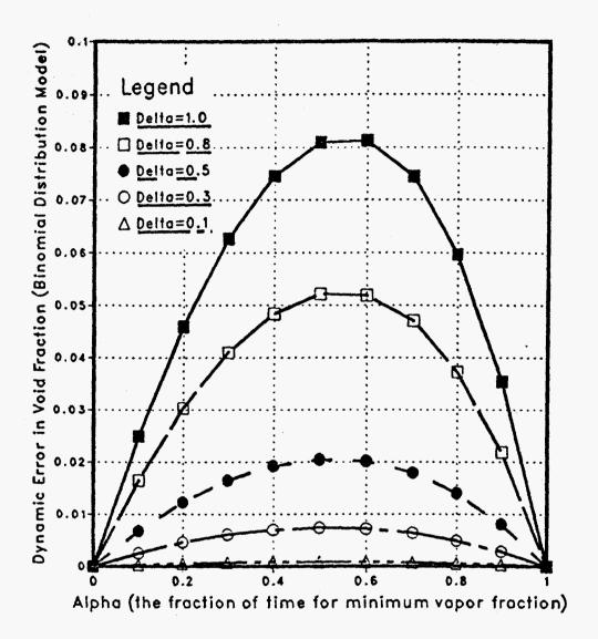
Delta = fluctuation in local void fractions during a measurement period = maximum void fraction - minimum void fraction
