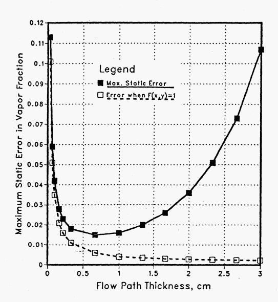
\* The attenuation coefficient of water used was 3.0 cm<sup>-1</sup>, and other data were based on specifications of the Penn State reactor facility. The maximum static error occurs when the vapor fraction becomes zero.
