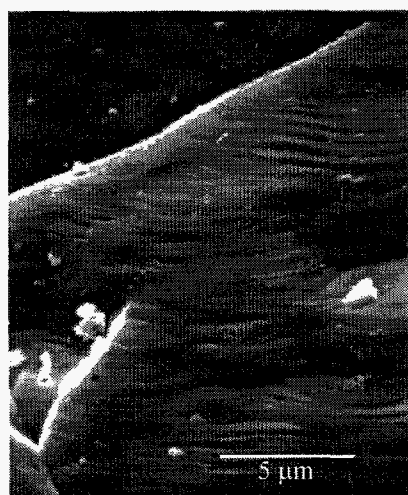
FIGURE 2. Electron Micrograph of an Alumina Sample after Diffusion Mode Exposure (6000X).
