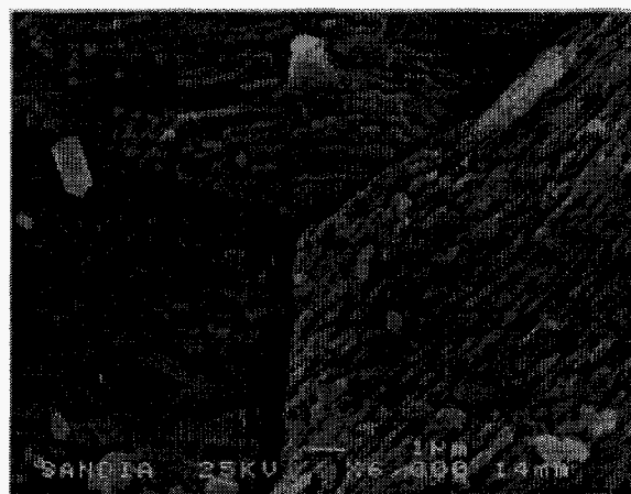
FIGURE 3. Electron Micrograph of an Alumina Sample near a Ta Retaining Strap after Diffusion Mode Exposure (6000X).
