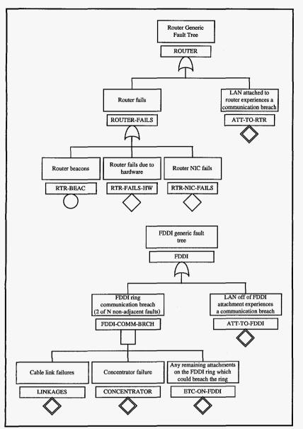
Figure 1. Example Generic Fault Tree Modules.
