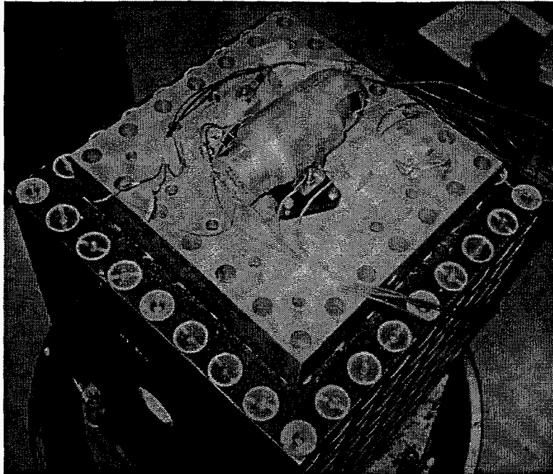
Figure 3: Weapon Component on Shaker Table
