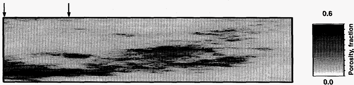
Figure 7. Cross section showing simulated stochastic artifacts that appear as high-porosity rock units in geologically unreasonable positions in the right-hand three-quarters of the figure. Geology consists of horizontal, alternating low-high-low porosity units as represented on the left-hand portion of the figure. Arrows indicate positions of conditioning drill holes. From information in Rautman and Robey, 1993.
