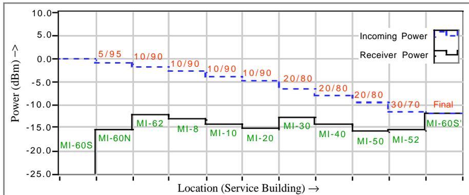
**FIGURE 2.** The passive splitting of a signal at each of the 10 service buildings. The top numbers indicate the splitter ratio while the top (dotted) line is the optical power in the incoming fiber to the service building. The lower (solid) line is the optical power to the receivers at each location with the name of the service building below the solid line. This calculation assumes a 1 dBm transmitter with a minimum receiver power requirement of -16 dBm.
