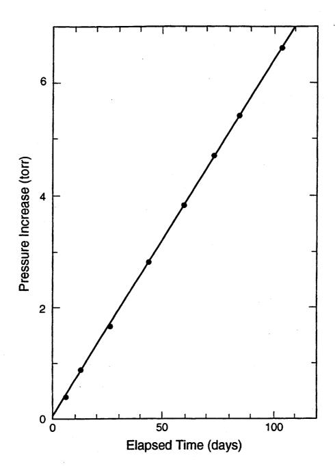
Figure 1. Time dependence of the pressure change during exposure of  $PuO_2$  to  $D_2O$  at 24.5°C and an initial pressure of 16.8 torr.
