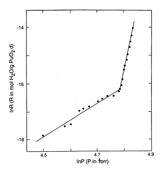
Figure 3. Dependence of lnR on lnP for the H<sub>2</sub>+O<sub>2</sub> reaction during exposure of PuO<sub>2</sub> to a 2:1 D<sub>2</sub>:O<sub>2</sub> mixture at 24.5°C. Values of R and P are listed in Table 1.
