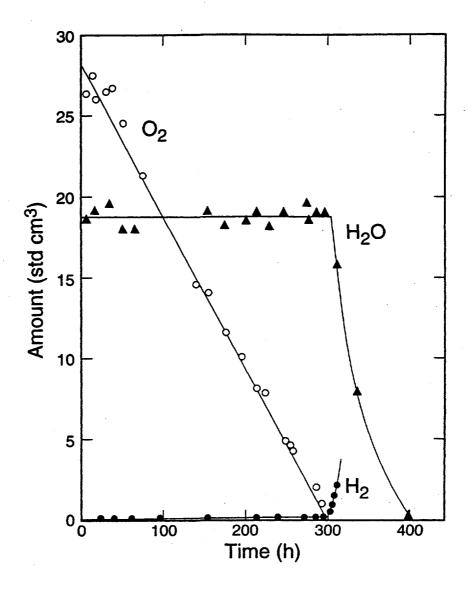
Figure 4. Time dependence of constituents in the gas phase during reaction of uranium metal with a 3:2 O<sub>2</sub>:H<sub>2</sub>O mixture at 100°C. The data are from the report by McD. Baker, Ness, and Orman (Reference 24).
