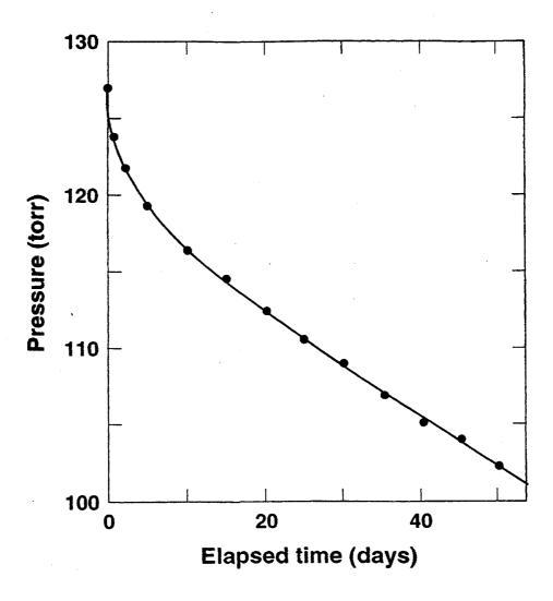
Figure 2. Time dependence of the pressure during exposure of PuO<sub>2</sub> to a 2:1 D<sub>2</sub>:O<sub>2</sub> mixture at 24.5°C and an initial pressure of 126.7 torr.
