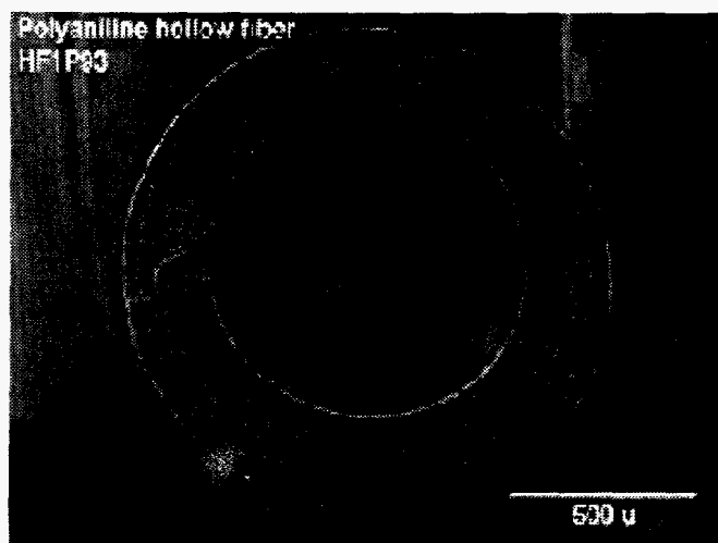
Figure 1. Four patented geometries of the electrically conducting polymer polyaniline were developed: (a) engineered porous flat sheet membranes, (b) barrier coatings, (c) engineered porous and integrally skinned asymmetric hollow fibers, and (d) electrically conductive solid fibers (clockwise from top left to bottom right.)
