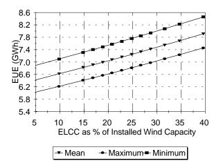
Figure 8. Reliability curves within one standard deviation of the mean ELCC value
