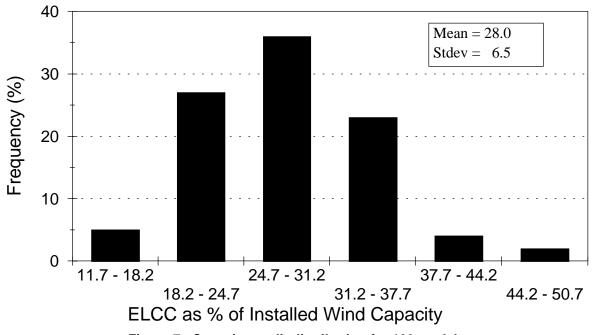
Figure 7. Capacity credit distribution for 100 model runs
