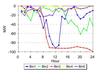
Figure 15. Reduction in base and intermediate generation, REPA cases, October 14
