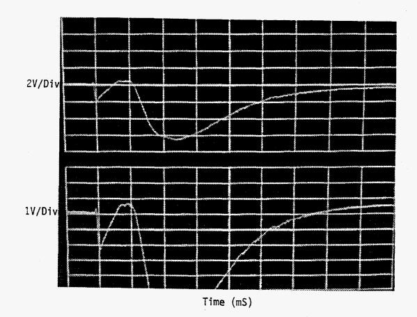
Figure 1. This is is the signal from the firing of a military rifle. Both traces are the same signal but recorded at different amplitudes.
