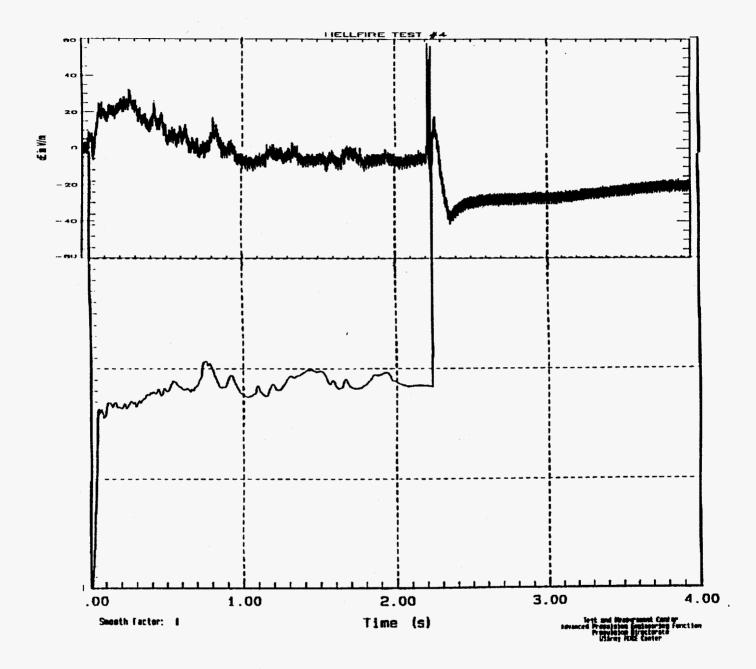
Figure 3. Data from anti-tank rocket motor. Top trace is the electric field and the bottom trace is the thrust. Rocket exploded at 2.2 seconds.
