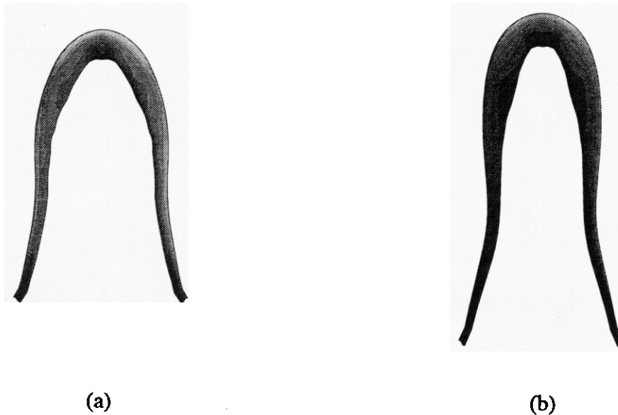
Figure 1: Comparison of projectile shape and fringes of plastic strain using the MTS model (a) and the previously “calibrated” Zerilli-Armstrong model (b). The black fringe level is plastic strain greater than 200% while white is less than 100%.
