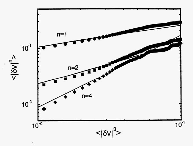
Fig. 2. Single-point velocity correlation functions < |dv|n> vs < |dv|3>showing the property of "Extended Self-Similarity" in thermal convection.
