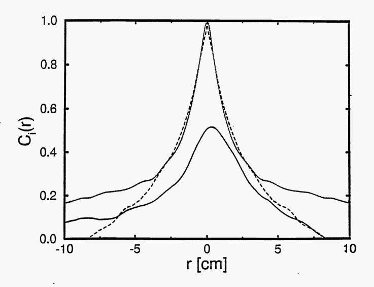
Fig. 1. Correlation functions of temperature (dashed line) and velocity (dotted line) and temperature-velocity (solid line) showing strong correlation between the two fields. This correlation demonstrates that for length scales larger than the Bolgiano length, temperature in convection is not a passive scalar field.
