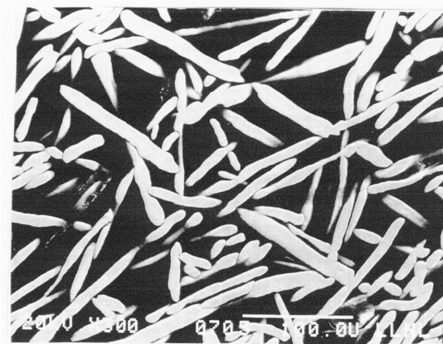
Figure 23. Electron micrograph of a cross section of a steel fibrous filter in a plane perpendicular to the air flow.
