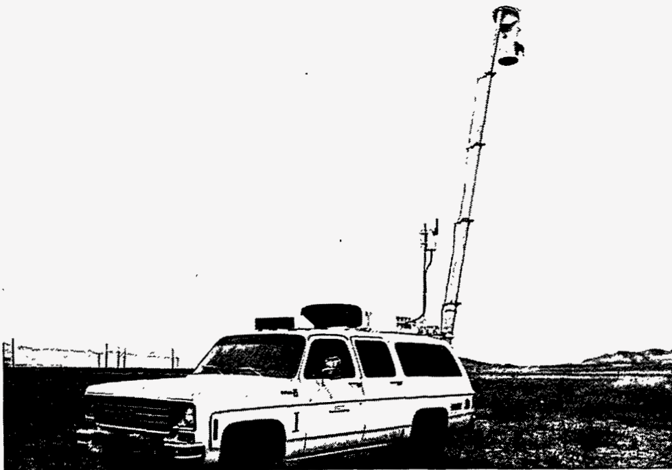
FIGURE 1. SUBURBAN VEHICLE WITH HPGe DETECTOR ON MAST. The detector on the end of the mast can be extended up to 7.5 m above the ground.
