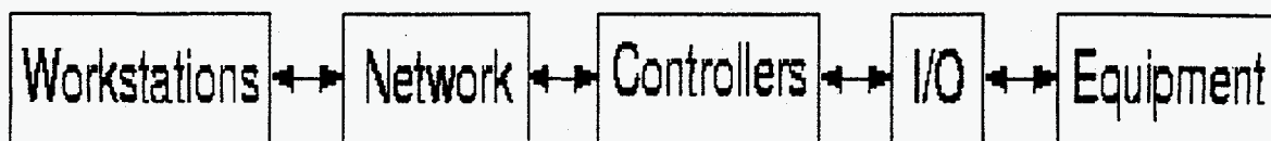
Figure 7 EPICS: control system architecture for the 90's
