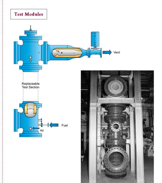
Refractory-lined test modules with multiple ports for temperature and pressure measurement as well as optical diagnostics
