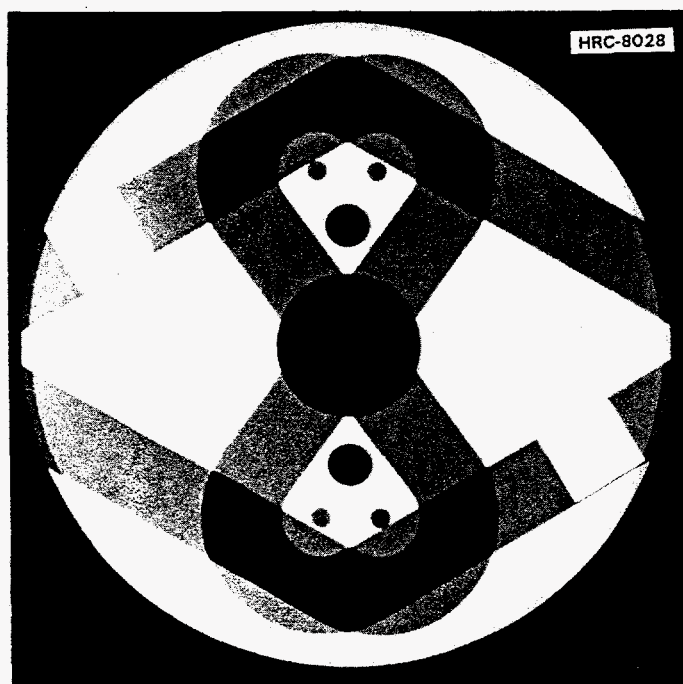
Fig. 6. Radiograph of HOM Suppression Circuit Cold Test Model Showing the 4-Port Folded Waveguide Concept.
