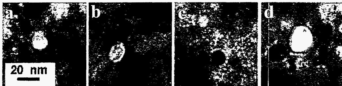
Fig. 1. Underfocused TEM images of craters resulting from impacts of Au with individual heavy ions: a) 200 keV Xe + , b) 200 keV Kr + , c) 200 keV Au + , d) 600 keV Au + .
