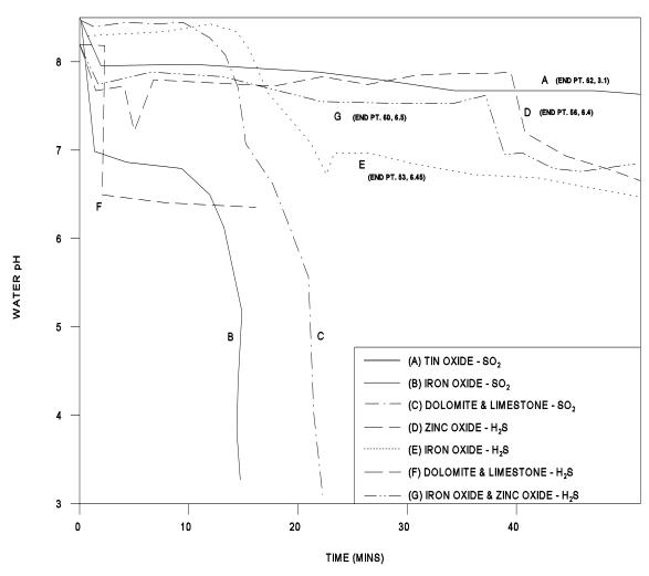
BREAKTHROUGH CURVES AT AMBIENT TEMPERATURE: pH vs. ELAPSED TIME
