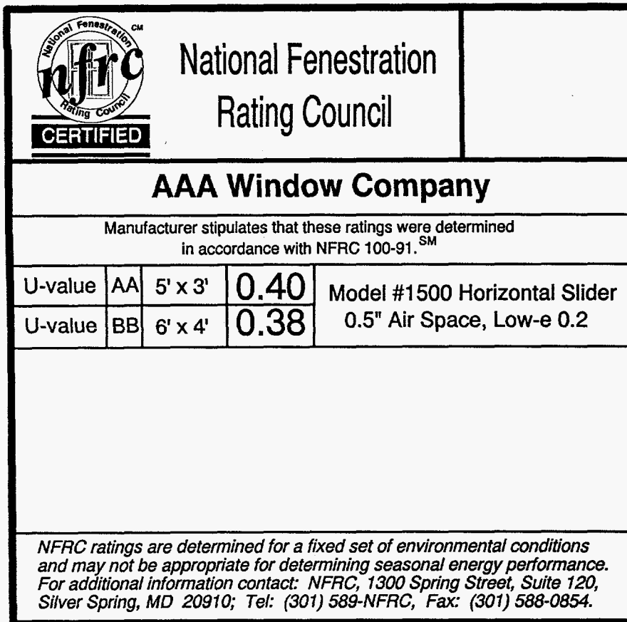
Figure 5. Sample NFRC label showing U-value data for two standard window sizes.
