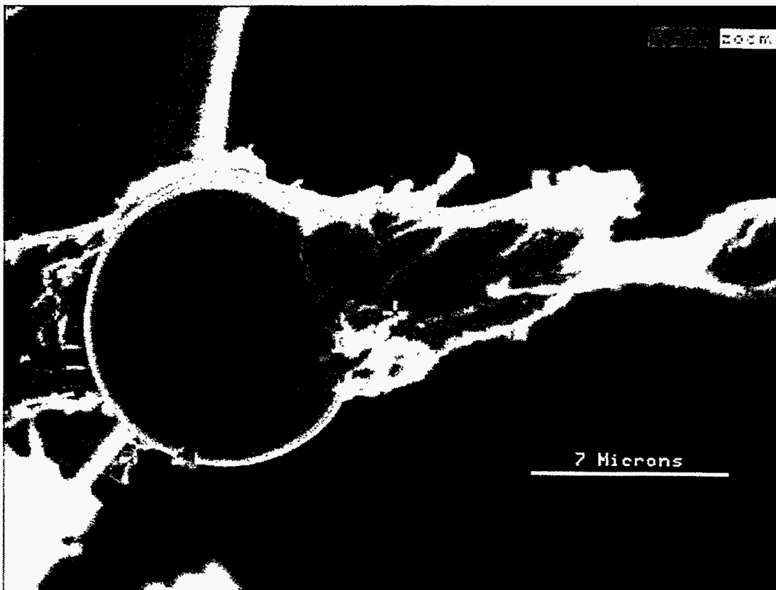
Fig. 12. SEM images of calcite and opal-A mineralization in a fossil root from 42 ft depth in the northern part of Pit 39 (sample F61, backscattered-electron images). Calcite fibers typically have tapered terminations and rugose surfaces. Opal-A occurs as small spherules, often precipitated on previously formed calcite fibers.
