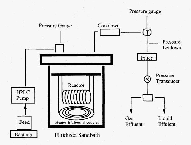
FIGURE 1: Schematic of tubular flow reactor
