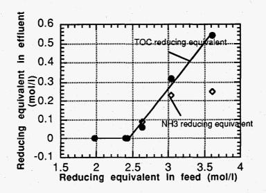
FIGURE 5: Ammonia and carbon reducing equivalent concentrations in effluent for 1 mol/l ammonium nitrate with phenol at 500 °C and 345 bar
