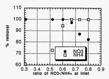
FIGURE 2: Ammonia and nitrate removal for the oxidation of ammnonia by nitrate (0.5 mol/l) at 500 °C and 375 bar
