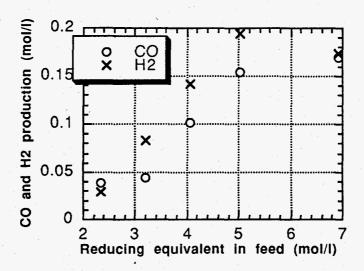
FIGURE 6: Hydrogen and Carbon Monoxide concentrations in effluent for 1 mol/l ammonium nitrate with methanol at 500 °C and 345 bar
