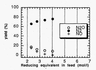
FIGURE 10: Yield of N<sub>2</sub>, N<sub>2</sub>O and NO for 1 mol/l ammonium nitrate with acetic acid at 500 °C and 345 bar.
