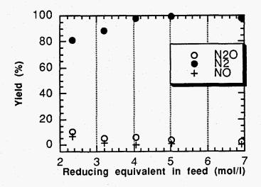
FIGURE 9: Yield of N<sub>2</sub>, N<sub>2</sub>O and NO for 1 mol/l ammonium nitrate with methanol at 500 °C and 345 bar.
