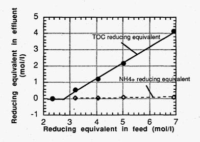
FIGURE 3: Ammonia and carbon reducing equivalent concentrations in effluent for 1 mol/l ammonium nitrate with methanol at 500 °C and 345 bar
