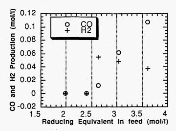
FIGURE 8: Hydrogen and Carbon Monoxide concentrations in effluent for 1 mol/l ammonium nitrate with acetic acid at 500 °C and 345 bar
