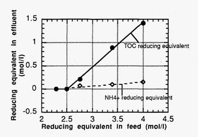
FIGURE 4: Ammonia and carbon reducing equivalent concentrations in effluent for 1 mol/l ammonium nitrate with acetic acid at 500 °C and 345 bar
