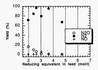
FIGURE 11: Yield of N2, N2O and NO for 1 mol/l ammonium nitrate with phenol at 500 °C and 345 bar.
