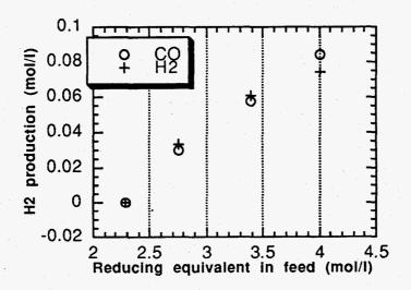
FIGURE 7: Hydrogen and Carbon Monoxide concentrations in effluent for 1 mol/l ammonium nitrate with acetic acid at 500 °C and 345 bar
