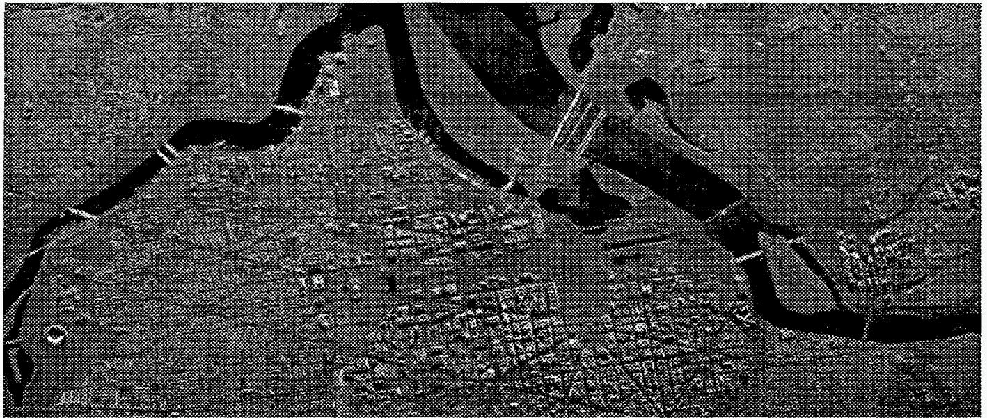
Figure 2. SAR Image of Washington, DC at 1-m Resolution, Ku Band
