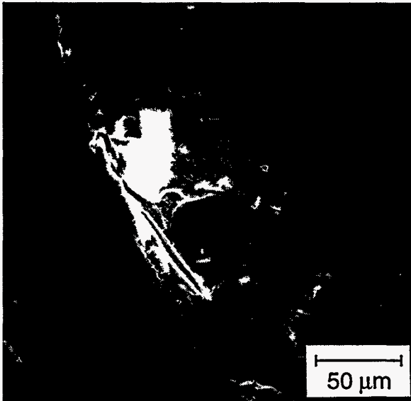
Figure 5. A portion of the surface of the void region in the slug is covered with a slag that has numerous cracks.
