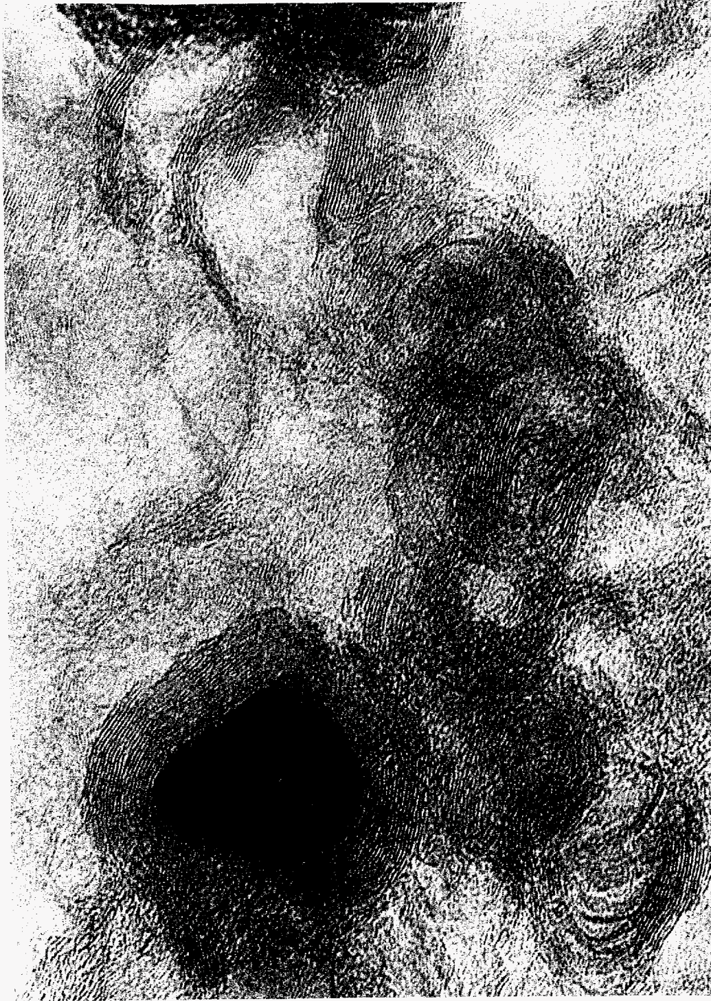
Figure 1.4 Development of concentric carbon crystalline structures in Fe-doped polyacrylonitrile carbon foam.† Iron inclusions are often seen to be the nucleus for growth of the concentric crystallites.
