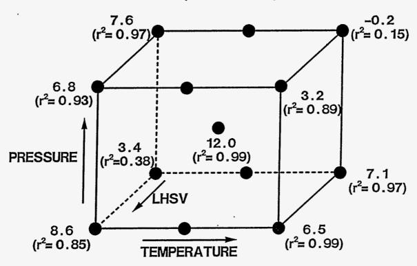
Figure 4: Measured and Calculated Nitrogen Values (At 28,000g Total Feed Processed)
