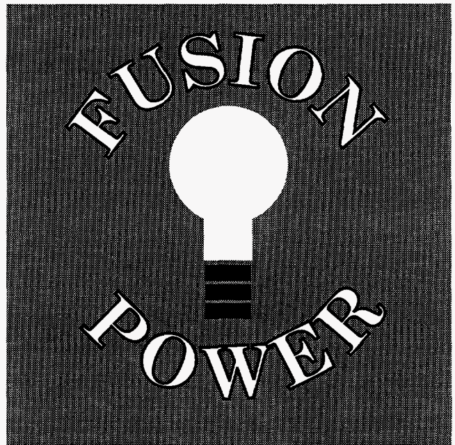
Figure 1. A TV monitor in the TFTR control room viewed this mask placed over a scintillator screen exposed to fusion neutrons near the TFTR machine. The brightness of the image provided scientists with instant feedback about the success or failure of the experiment.
