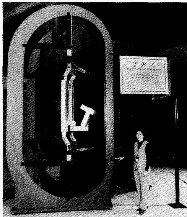
Figure 6. The basic TPX preliminary maintenance mock-up with a prototype maintenance vehicle installed. (95E0491)
