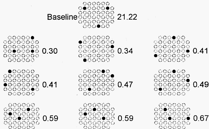
Figure 21 GA optimized designs and their transmissibilities at 50 Hz (in \mu\text{in/sec/lb} ), compared to baseline configuration.
