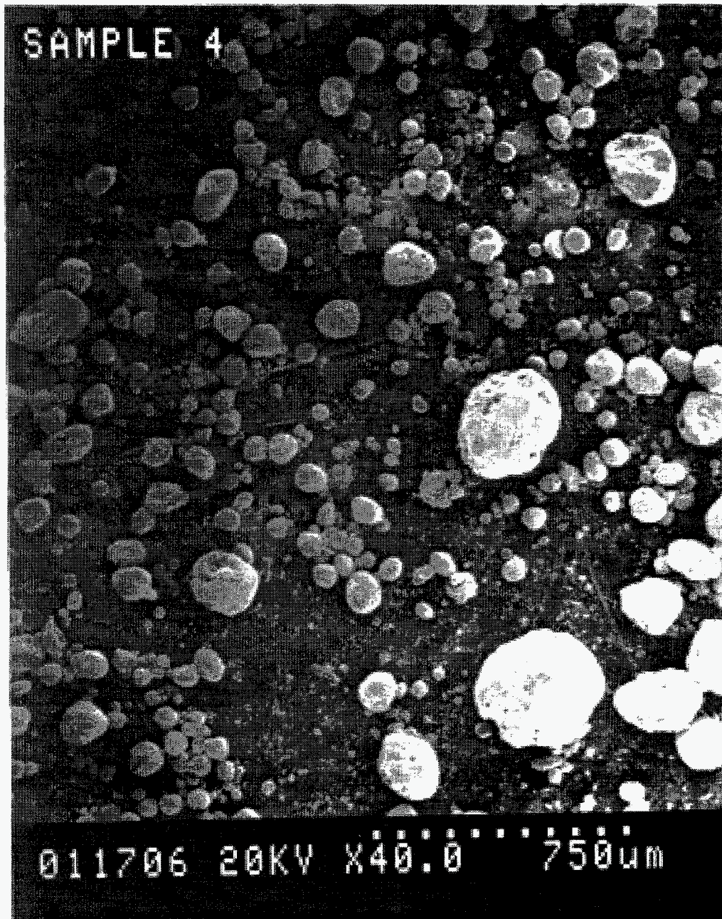
Figure E-4 SEM of Sludge A (750 \mu\text{m} magnification)
