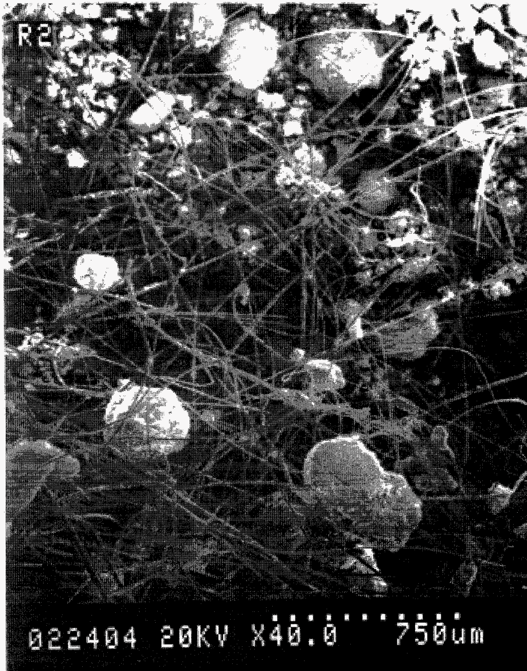
Figure E-23 SEM of a Typical Mixed Debris Bed (750 \mu\text{m} magnification)
