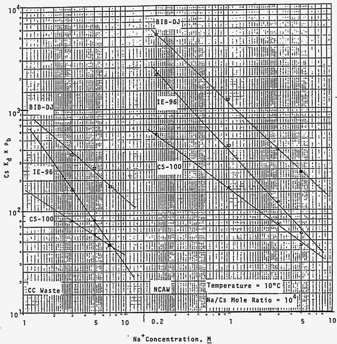
FIGURE 4. Effect of  $[Na^+]$  in CC and NCAW on performance of Ion Exchangers at  $10^\circ C$
