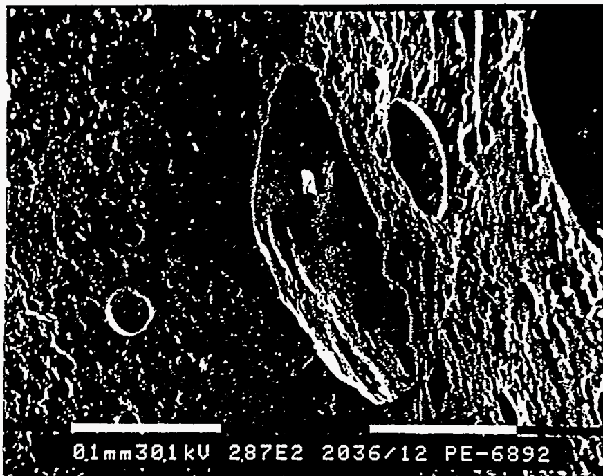
Fig.4 Rough fracture surface due to many inclusions
