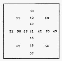
Figure 1 - Sample Results (in micrograms/gram of filter paper) for the First Stage HEPA filter - Air Inlet
