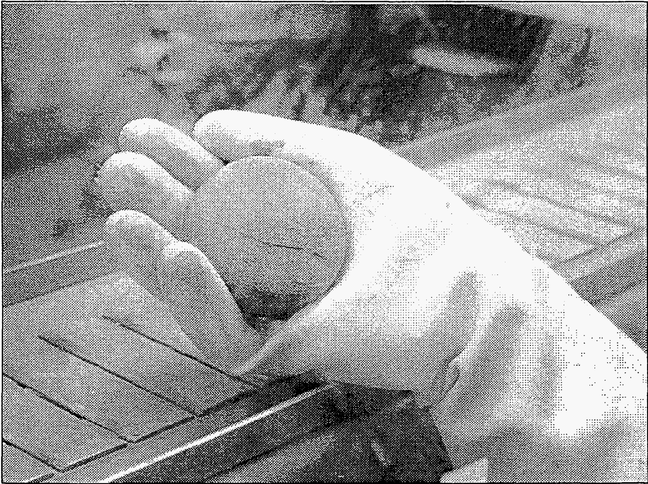
Figure 3 Two kilogram plutonium metal button shown shortly after being produced in 1988.
