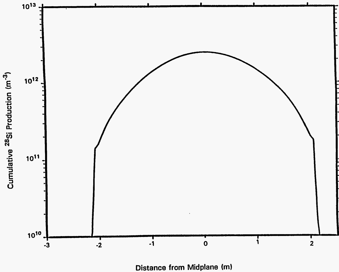
Fig. 7.25. ANS ^{28}\text{Si} production in the reflector vessel wall per cycle.
