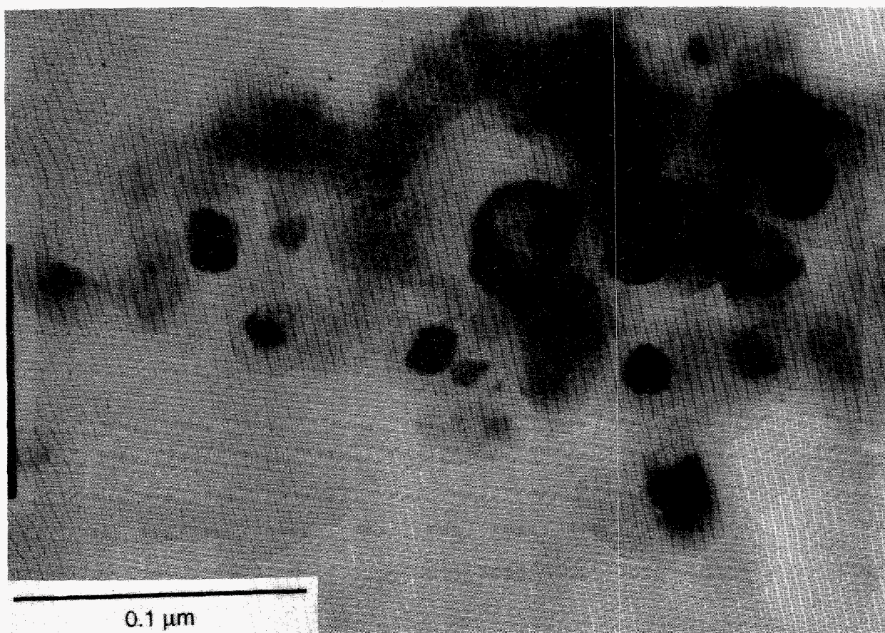
Figure 3. TEM of carbon coated TiO 2 precursor by the pyrolysis of C 3 H 6 at 600°C.
