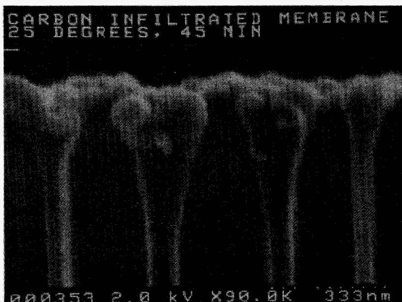
Figure 8. Pore tapering by magnetron sputtering of carbon
