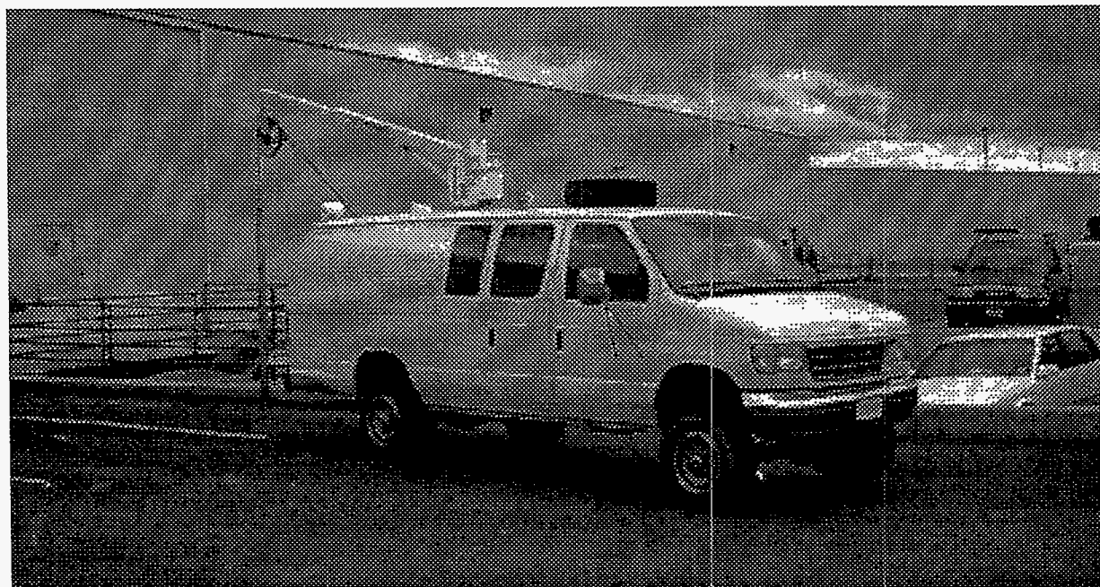
Figure 2. Gamma Spectroscopy Logging System with logging tool.
