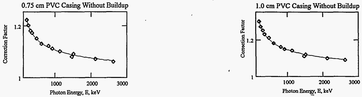
Figure 16. PVC casing correction factors for casing thicknesses of 0.75-cm and 1.0-cm.
